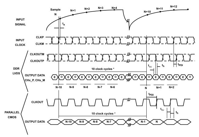
1) ADC latency after reset, At higher sampling frequencies, t<sub>PDI</sub> > 1 clock cycle which then makes the overall latency = ADC latency + 1. 2) E – Even bits D0, D2, D4..., O – Odd bits D1, D3, D5...
