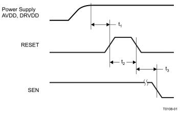
NOTE: A high-going pulse on RESET pin is required in serial interface mode in case of initialization through hardware reset.
