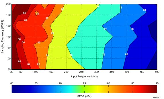
SFDR vs INPUT FREQUENCY AND SAMPLING FREQUENCY
