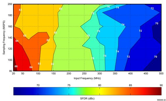
SFDR vs INPUT FREQUENCY AND SAMPLING FREQUENCY
