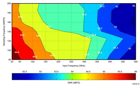
SNR vs INPUT FREQUENCY AND SAMPLING FREQUENCY
