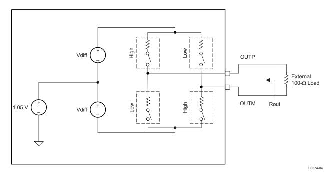
Figure 62. LVDS Buffer Equivalent Circuit
