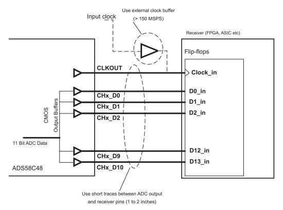
Figure 65. Data Capture with CMOS Interface
