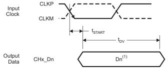
1. Dn - Bits D0,D1,D2... of channel A,B,C, and D
