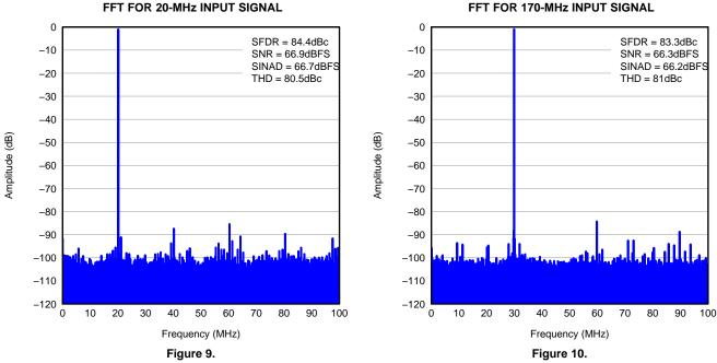
FFT FOR 170-MHz INPUT SIGNAL
