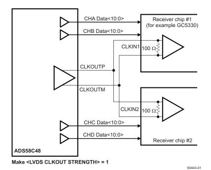
Figure 63. LVDS Strength Doubling - Example Application
