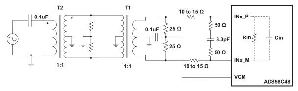
Figure 54. Drive Circuit with Low Bandwidth (For low input frequencies)
