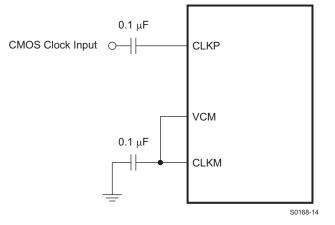
Figure 59. Single-Ended Clock Driving Circuit
