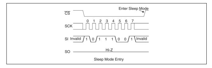
Returning to an normal operation from the SLEEP mode is carried out after  $t_{REC}$  (Max 400  $\mu$ s) time from the falling edge of  $\overline{CS}$  (see the <u>fig</u>ure below). It is possible to return  $\overline{CS}$  to H level before  $t_{REC}$  time. However, it is prohibited to bring down  $\overline{CS}$  to L level again during  $t_{REC}$  period.
