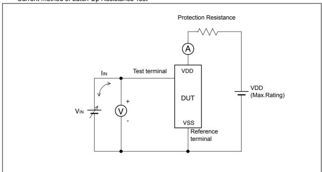
Note: The voltage  $V_{IN}$  is increased gradually and the current  $I_{IN}$  of 300 mA at maximum shall flow. Confirm the latch up does not occur under  $I_{IN} = \pm 300$  mA. In case the specific requirement is specified for I/O and  $I_{IN}$  cannot be 300 mA, the voltage shall be increased to the level that meets the specific requirement.
