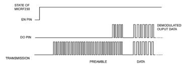
Figure 8. Preamble Length - Sufficient
