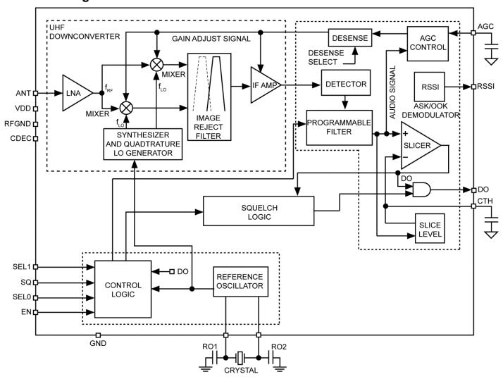
Figure 1. MICRF230 Simplified Functional Block Diagram
