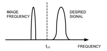
Figure 2. Low-Side Injection Local Oscillator
