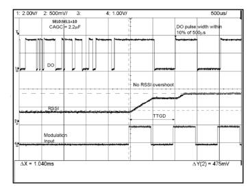
Figure 5. Proper TTGD (1ms) with Sufficient AGC
