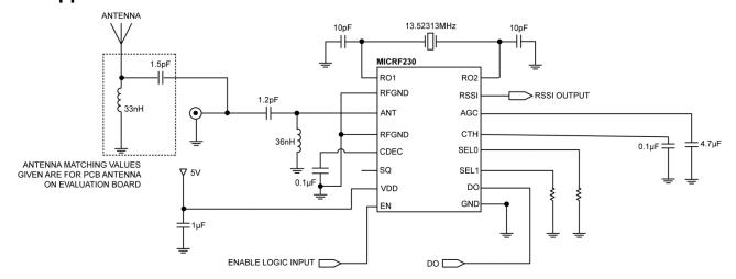
MICRF230 Typical Application Circuit for 433.92MHz
