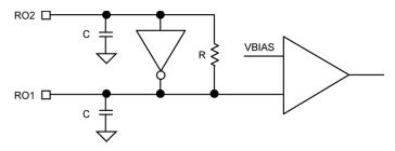
Figure 6. Reference Oscillator Circuit
