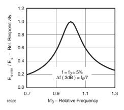
Figure 5. Frequency Dependence of Responsivity
