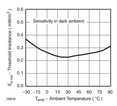
Figure 10. Sensitivity vs. Ambient Temperature
