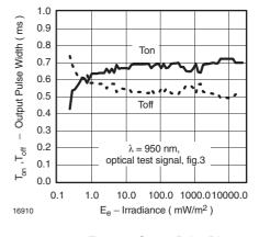
Figure 4. Output Pulse Diagram
