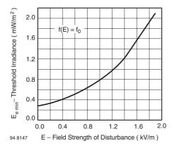
Figure 8. Sensitivity vs. Electric Field Disturbances
