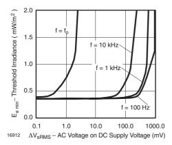
Figure 7. Sensitivity vs. Supply Voltage Disturbances
