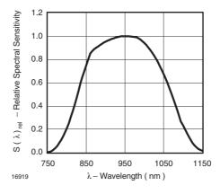
Figure 11. Relative Spectral Sensitivity vs. Wavelength
