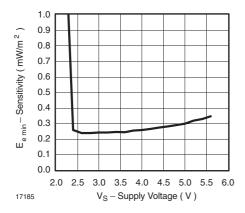
Figure 13. Sensitivity vs. Supply Voltage
