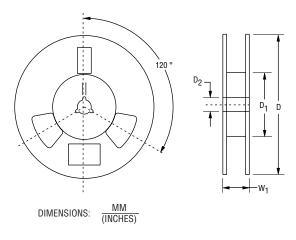
Devices are packed in accordance with EIA standard EIA-481-D and specifications shown here.
