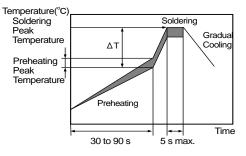
[Allowable Flow Soldering Temperature and Time]
