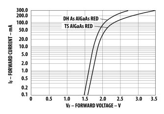
Figure 2. Forward current vs. forward voltage (non-resistor lamp).
