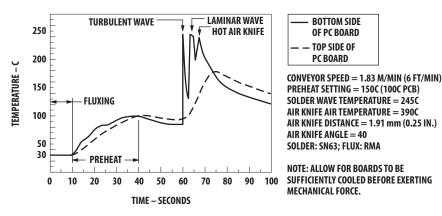
Figure 8. Recommended wave soldering profile.
