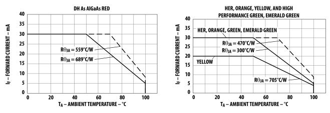
Figure 5. Maximum forward dc current vs. ambient temperature. Derating based on  $T_iMAX = 110$  °C.
