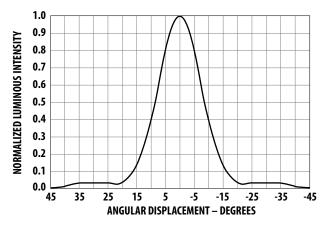
Figure 6. Relative luminous intensity vs. angular displacement. 15 degree family.
