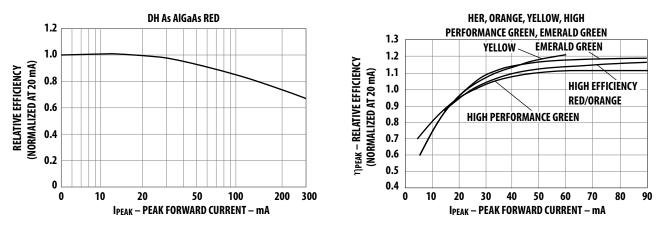
Figure 4. Relative efficiency (luminous intensity per unit current) vs. peak current.
