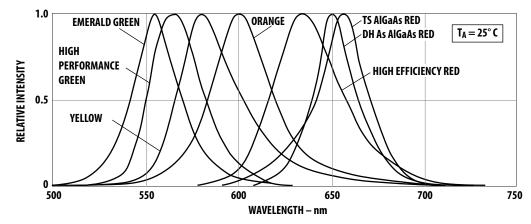
Figure 1. Relative intensity vs. wavelength.
